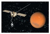
A MARSIS satellite nears Mars, showing one composite antenna boom already deployed and a second boom in the process of unfolding. Image courtesy European Space Agency.
